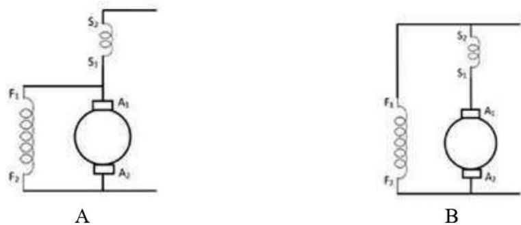
Fig. 1.19 A A Schematic diagram of short -shunt compound machine
