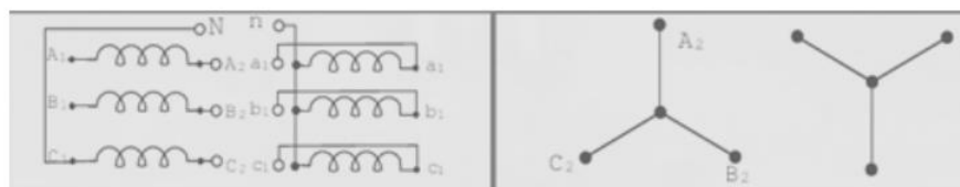
Fig 4.13. Yy6 connection and phasor diagram
